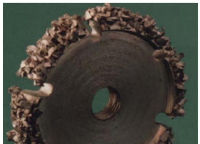
Specimen of an abrasive tool (Innobraze GmbH, Esslingen)
